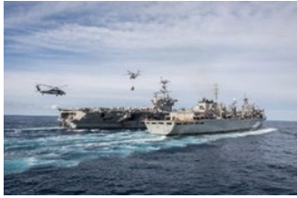
Supply-class fast combat support ship USNS Supply (T-AOE-6), right, replenishing U.S. Navy Nimitz-class aircraft carrier USS Harry S. Truman, left. Photo credit: Petty Officer Marius Vaagenes Villanger / Norwegian Armed Forces.
